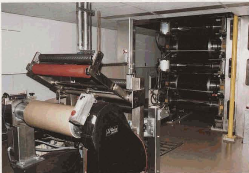
PERKINS, MRD, AND PASSAVANT MULTIPLE ROLL VERTICAL (4) AND HORIZONTAL (1) CALENDARS. OVER 70 COMPLIANT AND CHROMED STEEL SPARE ROLLS AVAILABLE
