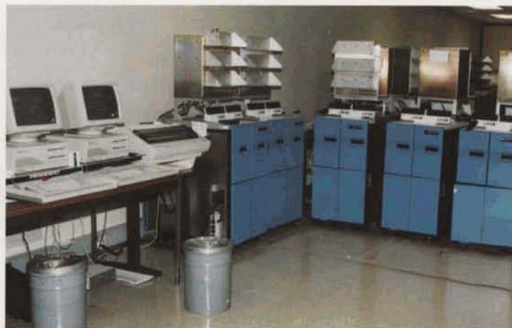
OVER 30 CARTRIDGE TESTERS INCLUDING IBM 3840, FUJITSU 5480 AND 5481; OVER 20 CTC-1 SINGLE AND DUAL CERTIFIERS
