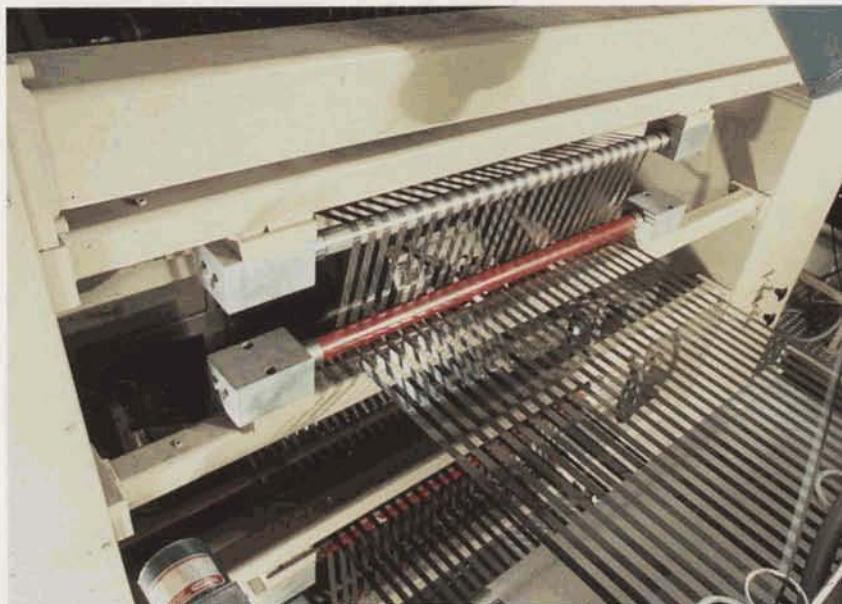
THREE DUSENBURY SLITTING MACHINES FOR CUTTING 26" WEBS, UP TO 40K FEET, THICKNESS 0.25 MIL TO 1.5 MIL
